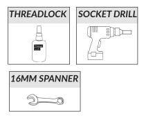
We strongly recommend applying thread lock to ends of the booker rod and using an socket drill.
